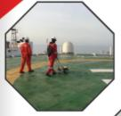
Offshore Helideck and Onshore Elevated Heliport Surface Friction Testing, Using the Findlay Irvine Micro GT Helideck Friction Tester
